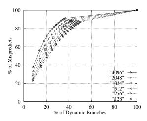
Fig. 10. Performance with small CIR tables; tables hold resetting counters, accessed with PC xor BHR.
