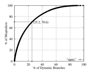
Fig. 2. Cumulative mispredictions versus cumulative dynamic branches.
