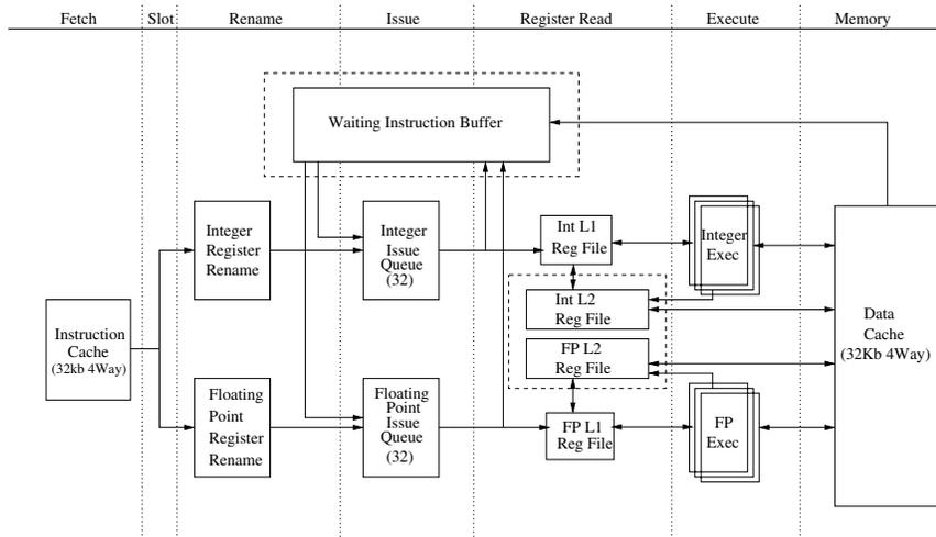
**Figure 2. WIB-based Microarchitecture**
