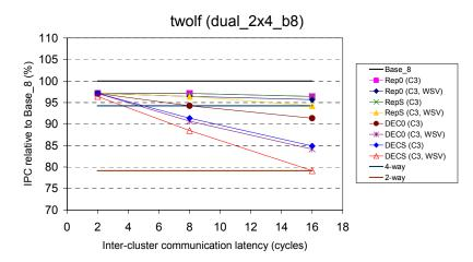
Figure A-7: Relative performance of slipstream-based steering (confidence threshold of 3) on dual 2x4 b8, with respect to Base 8, for *twolf*.
