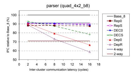
Figure 6-36: Relative performance of slipstream-based steering (confidence threshold of 15 and no WSV) and dependence-based steering on quad\_4x2\_b8, with respect to Base\_8, for *parser*.
