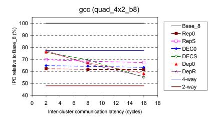
Figure 6-34: Relative performance of slipstream-based steering (confidence threshold of 15 and no WSV) and dependence-based steering on quad\_4x2\_b8, with respect to Base\_8, for *gcc*.
