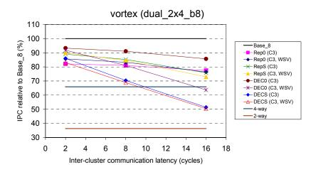
Figure A-9: Relative performance of slipstream-based steering (confidence threshold of 3) on dual\_2x4\_b8, with respect to Base\_8, for *vortex*.
