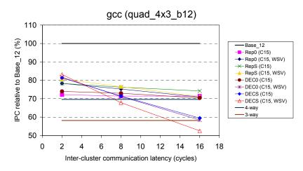
Figure A-14: Relative performance of slipstream-based steering (confidence threshold of 15) on quad\_4x3\_b12, with respect to Base\_12, for gcc.
