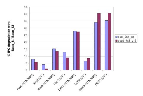
Figure 6-43: Relative performance degradation of slipstream-based algorithms for dual\_2x4\_b8 and quad\_4x3\_b12, for *vortex*.
