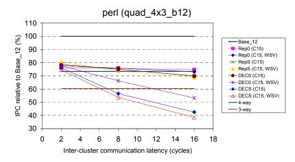
Figure A-16: Relative performance of slipstream-based steering (confidence threshold of 15) on quad 4x3 b12, with respect to Base 12, for *perl*.
