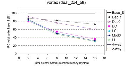
Figure 6-5: Relative performance of conventional steering on dual\_2x4\_b8, with respect to Base\_8, for *vortex*.
