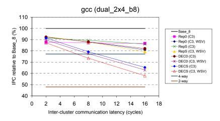
Figure A-3: Relative performance of slipstream-based steering (confidence threshold of 3) on dual\_2x4\_b8, with respect to Base\_8, for *gcc*.
