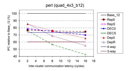
Figure 6-49: Relative performance of slipstream-based steering (confidence threshold of 15 and no WSV) and dependence-based steering on quad\_4x3\_b12, with respect to Base\_12, for *perl*.
