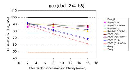
Figure A-4: Relative performance of slipstream-based steering (confidence threshold of 15) on dual 2x4 b8, with respect to Base 8, for gcc.
