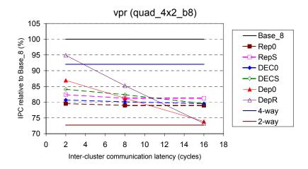
Figure 6-40: Relative performance of slipstream-based steering (confidence threshold of 15 and no WSV) and dependence-based steering on quad\_4x2\_b8, with respect to Base\_8, for *vpr*.
