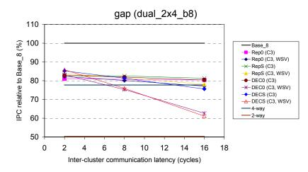
Figure A-1: Relative performance of slipstream-based steering (confidence threshold of 3) on dual 2x4 b8, with respect to Base 8, for *gap*.
