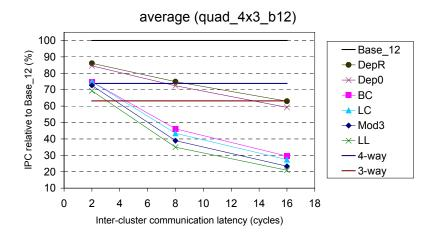
Figure 6-19: Relative performance of conventional steering on quad\_4x3\_b12, with respect to Base\_12. Results are averaged across five benchmarks.
