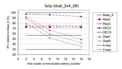
Figure 6-21: Relative performance of slipstream-based steering (confidence threshold of 15 and no WSV) and dependence-based steering on dual\_2x4\_b8, with respect to Base\_8, for *bzip*.
