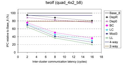
Figure 6-11: Relative performance of conventional steering on quad\_4x2\_b8, with respect to Base\_8, for *twolf*.
