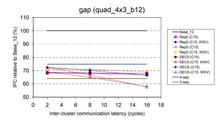
Figure A-13: Relative performance of slipstream-based steering (confidence threshold of 15) on quad\_4x3\_b12, with respect to Base\_12, for *gap*.
