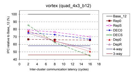
Figure 6-51: Relative performance of slipstream-based steering (confidence threshold of 15 and no WSV) and dependence-based steering on quad 4x3 b12, with respect to Base 12, for *vortex*.
