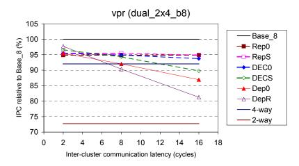
Figure 6-29: Relative performance of slipstream-based steering (confidence threshold of 15 and no WSV) and dependence-based steering on dual\_2x4\_b8, with respect to Base\_8, for *vpr*.
