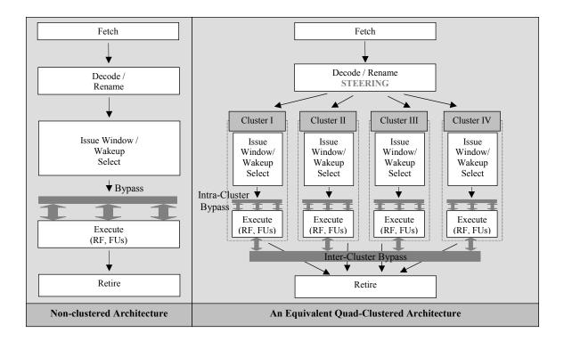
Figure 2-1: Comparison between a non-clustered microarchitecture and a quad-clustered microarchitecture.
