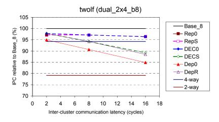
Figure 6-27: Relative performance of slipstream-based steering (confidence threshold of 15 and no WSV) and dependence-based steering on dual\_2x4\_b8, with respect to Base\_8, for *twolf*.
