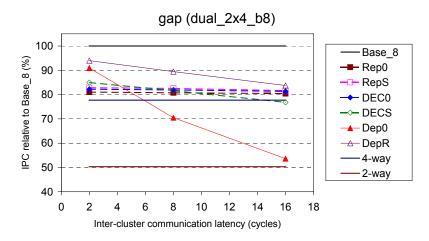
Figure 6-22: Relative performance of slipstream-based steering (confidence threshold of 15 and no WSV) and dependence-based steering on dual 2x4 b8, with respect to Base 8, for *gap*.
