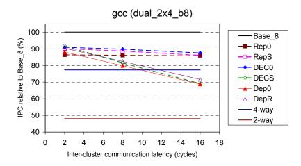
Figure 6-23: Relative performance of slipstream-based steering (confidence threshold of 15 and no WSV) and dependence-based steering on dual\_2x4\_b8, with respect to Base\_8, for *gcc*.
