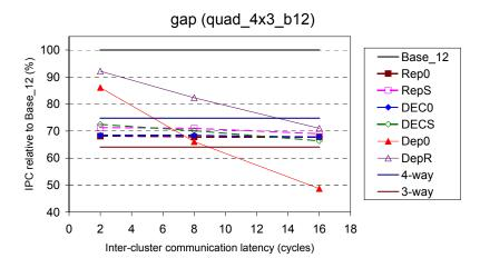
Figure 6-45: Relative performance of slipstream-based steering (confidence threshold of 15 and no WSV) and dependence-based steering on quad 4x3 b12, with respect to Base 12, for *gap*.
