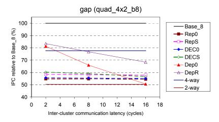
Figure 6-33: Relative performance of slipstream-based steering (confidence threshold of 15 and no WSV) and dependence-based steering on quad 4x2 b8, with respect to Base 8, for *gap*.
