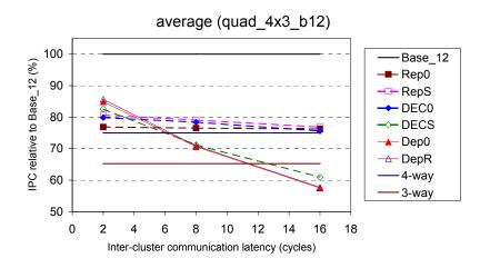
Figure 6-53: Relative performance of slipstream-based steering (confidence threshold of 15 and no WSV) and dependence-based steering on quad\_4x3\_b12, with respect to Base\_12. Results are averaged across all benchmarks.
