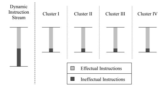
Figure 1-1: Replication model of instruction execution in a clustered microarchitecture.
