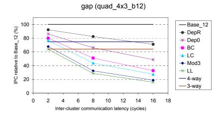
Figure 6-14: Relative performance of conventional steering on quad\_4x3\_b12, with respect to Base\_12, for *gap*.
