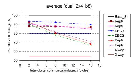
Figure 6-30: Relative performance of slipstream-based steering (confidence threshold of 15 and no WSV) and dependence-based steering on dual\_2x4\_b8, with respect to Base\_8. Results are averaged across all benchmarks.
