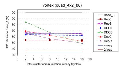
Figure 6-39: Relative performance of slipstream-based steering (confidence threshold of 15 and no WSV) and dependence-based steering on quad 4x2 b8, with respect to Base 8, for *vortex*.
