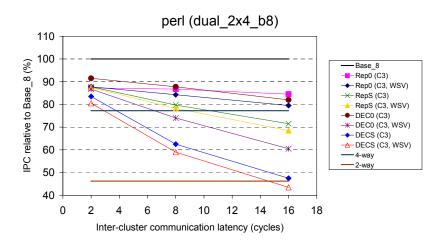
Figure A-5: Relative performance of slipstream-based steering (confidence threshold of 3) on dual\_2x4\_b8, with respect to Base\_8, for *perl*.
