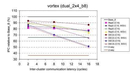
Figure A-10: Relative performance of slipstream-based steering (confidence threshold of 15) on dual 2x4 b8, with respect to Base 8, for *vortex*.
