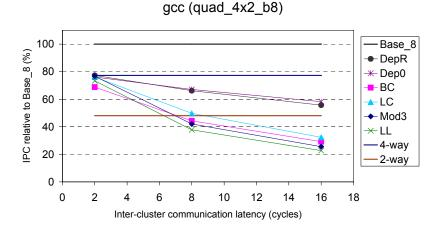
Figure 6-9: Relative performance of conventional steering on quad\_4x2\_b8, with respect to Base\_8, for *gcc*.
