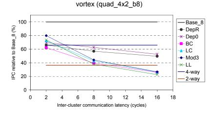
Figure 6-12: Relative performance of conventional steering on quad\_4x2\_b8, with respect to Base\_8, for *vortex*.
