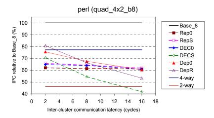
Figure 6-37: Relative performance of slipstream-based steering (confidence threshold of 15 and no WSV) and dependence-based steering on quad\_4x2\_b8, with respect to Base\_8, for *perl*.
