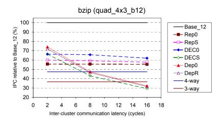
Figure 6-44: Relative performance of slipstream-based steering (confidence threshold of 15 and no WSV) and dependence-based steering on quad\_4x3\_b12, with respect to Base\_12, for *bzip*.
