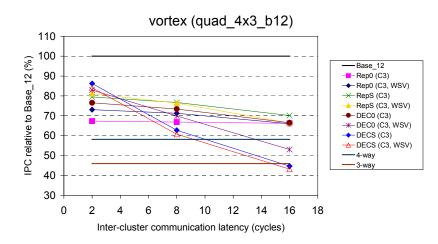
Figure A-17: Relative performance of slipstream-based steering (confidence threshold of 3) on quad\_4x3\_b12, with respect to Base\_12, for *vortex*.
