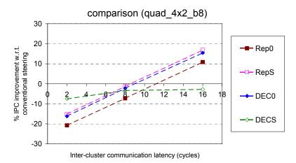
Figure 6-42: IPC improvement of slipstream-based steering (confidence threshold of 15 and no WSV) with respect to dependence-based steering on quad\_4x2\_b8. Results are averaged across all benchmarks.
