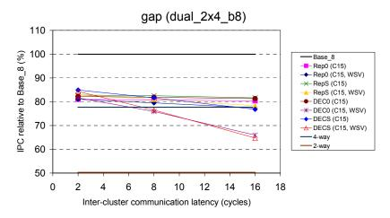
Figure A-2: Relative performance of slipstream-based steering (confidence threshold of 15) on dual\_2x4\_b8, with respect to Base\_8, for *gap*.
