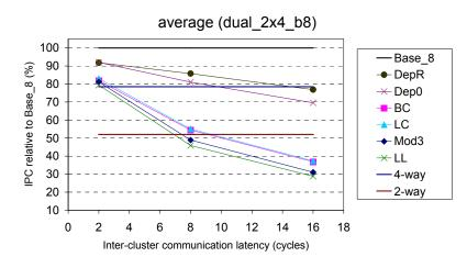
Figure 6-7: Relative performance of conventional steering on dual\_2x4\_b8, with respect to Base\_8. Results are averaged across five benchmarks.
