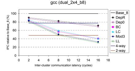
Figure 6-2: Relative performance of conventional steering on dual\_2x4\_b8, with respect to Base\_8, for *gcc*.
