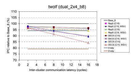
Figure A-8: Relative performance of slipstream-based steering (confidence threshold of 15) on dual\_2x4\_b8, with respect to Base\_8, for *twolf*.
