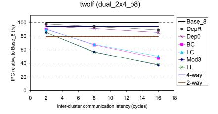
Figure 6-4: Relative performance of conventional steering on dual\_2x4\_b8, with respect to Base\_8, for *twolf*.
