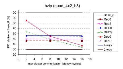
Figure 6-32: Relative performance of slipstream-based steering (confidence threshold of 15 and no WSV) and dependence-based steering on quad\_4x2\_b8, with respect to Base\_8, for *bzip*.
