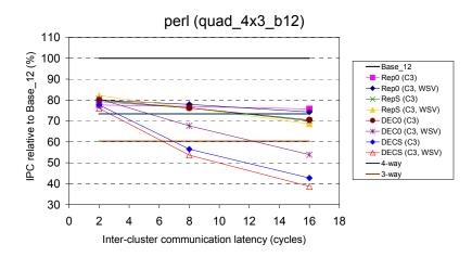
Figure A-15: Relative performance of slipstream-based steering (confidence threshold of 3) on quad\_4x3\_b12, with respect to Base\_12, for *perl*.
