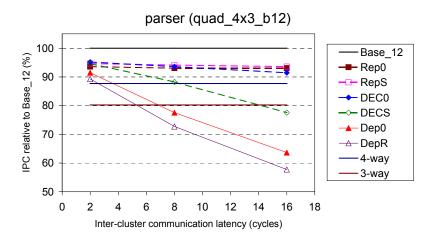
Figure 6-48: Relative performance of slipstream-based steering (confidence threshold of 15 and no WSV) and dependence-based steering on quad 4x3 b12, with respect to Base 12, for *parser*.
