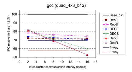
Figure 6-46: Relative performance of slipstream-based steering (confidence threshold of 15 and no WSV) and dependence-based steering on quad\_4x3\_b12, with respect to Base\_12, for *gcc*.
