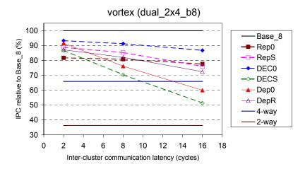
Figure 6-28: Relative performance of slipstream-based steering (confidence threshold of 15 and no WSV) and dependence-based steering on dual 2x4 b8, with respect to Base 8, for *vortex*.
