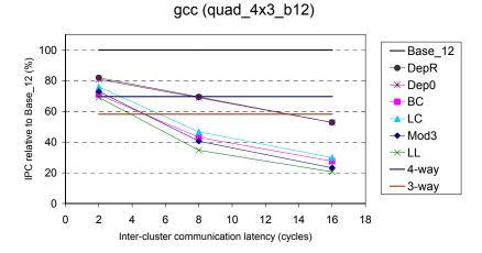
Figure 6-15: Relative performance of conventional steering on quad\_4x3\_b12, with respect to Base 12, for gcc.
