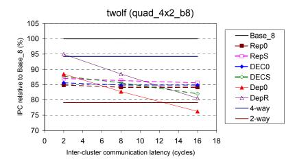
Figure 6-38: Relative performance of slipstream-based steering (confidence threshold of 15 and no WSV) and dependence-based steering on quad\_4x2\_b8, with respect to Base\_8, for *twolf*.
