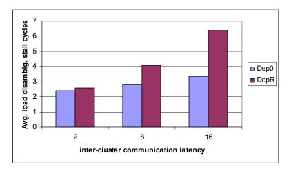
Figure 6-6: Average load disambiguation stall cycles of Dep0 and DepR on dual\_2x4\_b8, for perl.
