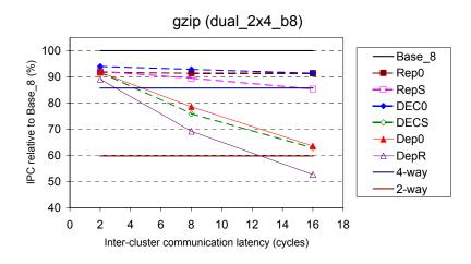
Figure 6-24: Relative performance of slipstream-based steering (confidence threshold of 15 and no WSV) and dependence-based steering on dual\_2x4\_b8, with respect to Base\_8, for *gzip*.
