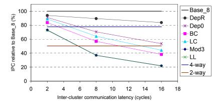
Figure 6-1: Relative performance of conventional steering on dual\_2x4\_b8, with respect to Base\_8, for *gap*.
