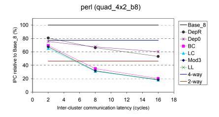
Figure 6-10: Relative performance of conventional steering on quad\_4x2\_b8, with respect to Base\_8, for *perl*.
