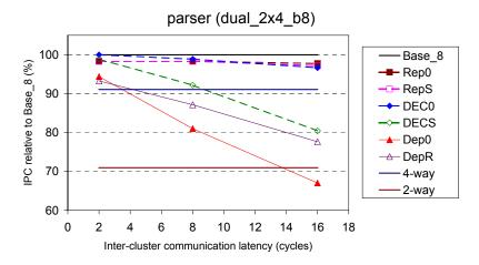
Figure 6-25: Relative performance of slipstream-based steering (confidence threshold of 15 and no WSV) and dependence-based steering on dual 2x4 b8, with respect to Base 8, for *parser*.
