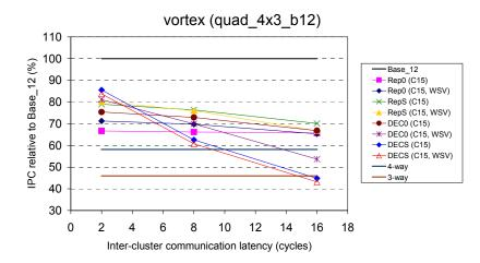
Figure A-18: Relative performance of slipstream-based steering (confidence threshold of 15) on quad\_4x3\_b12, with respect to Base\_12, for *vortex*.
