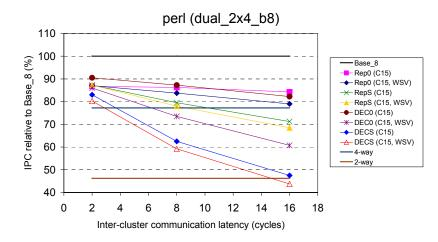
Figure A-6: Relative performance of slipstream-based steering (confidence threshold of 15) on dual\_2x4\_b8, with respect to Base\_8, for *perl*.
