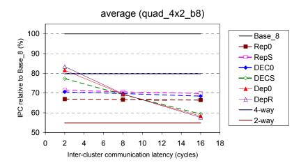
Figure 6-41: Relative performance of slipstream-based steering (confidence threshold of 15 and no WSV) and dependence-based steering on quad\_4x2\_b8, with respect to Base\_8. Results are averaged across all benchmarks.
