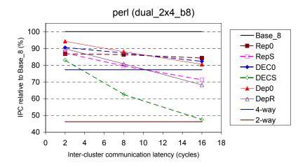
Figure 6-26: Relative performance of slipstream-based steering (confidence threshold of 15 and no WSV) and dependence-based steering on dual\_2x4\_b8, with respect to Base\_8, for *perl*.
