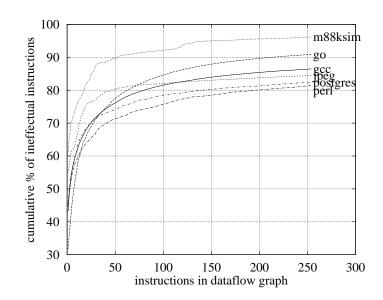
FIGURE 3. Size of dataflow graph and its impact on identification of ineffectual instructions.
