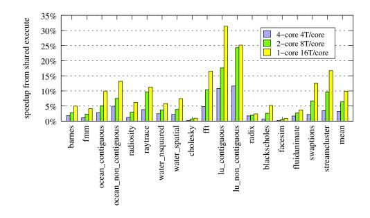
Fig. 9. Speedup of instruction sharing techniques on a 4-core/4-context-per-core processor, a 2-core/8-context-per-core processor, and a 1-core-16/contextper-core processor. Speedup is presented by comparing the throughput of each processor with shared execution enabled against each processor without shared execution. Match tables have 4 entries.
