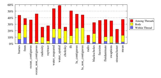
Fig. 5. The availability of matching instructions within a thread, among multiple threads, or both.
