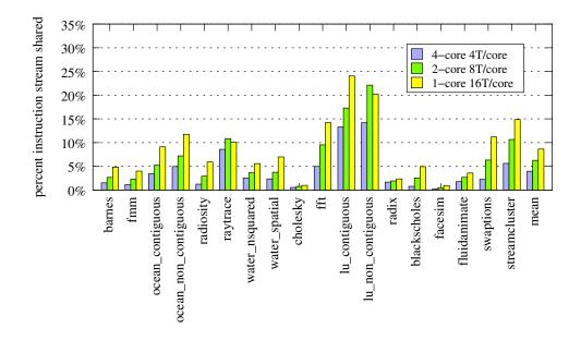
Fig. 10. Percent dynamic instruction stream shared using presented instruction sharing hardware on a 4-core/4-context-per-core processor, a 2-core/8-contextper-core processor, and a 1-core/16-context-per-core processor. Generally, the percent of the instruction stream shared correlates highly with the speedups obtained in Fig. 9. Match tables have 4 entries.
