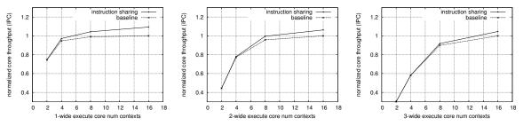
Fig. 1. Throughput impact of adding contexts to a 1-wide execute core, a 2-wide execute core, and a 3-wide execute core – both with and without multithreaded instruction sharing. Throughputs normalized to the 16-context baseline case.
