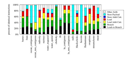
Fig. 4. Breakdown of shared instructions. The possible instruction types are based on either the instruction opcode, or the instructions dataflow contribution.
