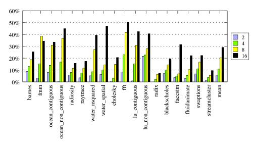
Fig. 3. Instruction matches when varying the number of threads while holding the buffer depth at a constant depth of 4. For each benchmark, the number of threads from left to right are 2, 4, 8, and 16.
