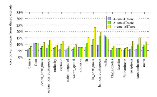
Fig. 11. Core power impact of implementing instruction sharing. Caches, interconnect, and memory controller power are excluded from this data. Power is increased by two sources. First, the additional register read process, and the match test and match table hardware contribute power. Second, by increasing performance, power demands on most core structures are also affected. E.g., by increasing fetch rate and IB write rates. Match tables have 4 entries.
