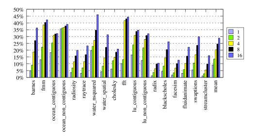
Fig. 2. Instruction matches when holding number of threads at 8 while varying the buffer depth. For each benchmark, the buffer depth from left to right is 1, 2, 4, 8, and 16.
