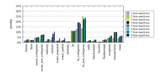
Fig. 13. Effect of limited match test. Instructions are only matched if they use source registers that contain sign-extended n-byte values. One additional bit is added to each register to indicate whether they meet this criteria. The sign extension bit and the lower bytes are tested instead of the full 64-bits.
