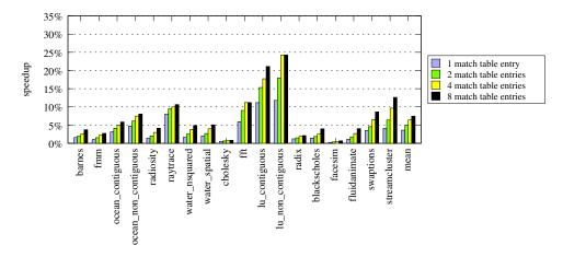
Fig. 12. Effects of various numbers of match table entries on the speedup afforded by instruction sharing. Match table entries are per-thread, as the processor maintains separate fully-associative match tables for each context. Data is presented for a 2-core/8-context-per-core processor.
