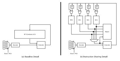
Fig. 7. (a) Detail of the baseline processor pipeline, illustrating portions of issue, decode, execute, and writeback. (b) Detail of proposed modifications to support instruction sharing. The monolithic register file has been split into context-specific register files. A match stage has been added to compare the contents of registers in each context for each issued instruction. Small fully-associative match tables have been added.
