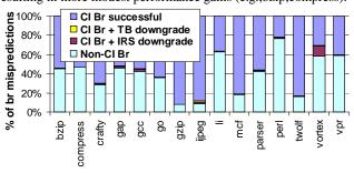
Figure 11. Breakdown of branch mispredictions.
