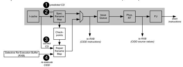
Figure 3. Transparent control independence (TCI) architecture.
