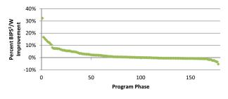
Fig. 13. Efficiency of each program phase for DC-T compared to heterogeneous core pair with coarse-grain migrations. TABLE II. PROTOTYPE CHIP CORES.
