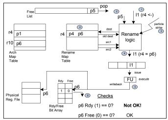
Figure 4. Fault detection using RNA-writeback.
