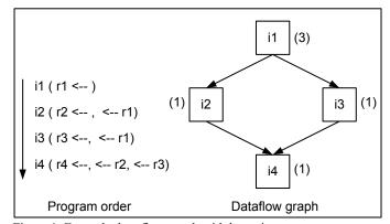
Figure 1. Example data-flow graph with latencies.
