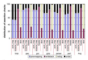
Figure 8. Relation of faults to assertion checks.
