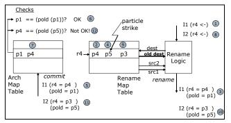
Figure 3. Fault detection using RNA's "previous mapping check".
