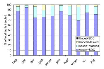
Figure 5. Breakdown of outcomes of TAC fault injection campaign.
