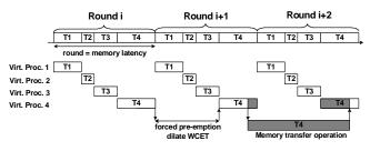
Figure 3. Exploiting WRR scheduling for bounding overlap.
