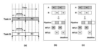
Figure 2. Overlapping execution of different task-sets on a multithreaded processor. (a) Task-set composed of tasks A and B (WCET<sub>A</sub>=period<sub>A</sub>=WCET<sub>B</sub>=period<sub>B</sub>). (b) A and B with two memory transfers each ("m") are schedulable because of computation-memory overlap. (c) B' is identical to B except for positioning of memory transfers, and is not schedulable with A.
